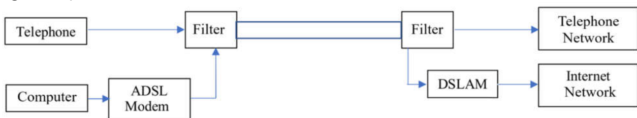
Figure III.4: ADSL link between an end-user and the voice and data networks.
